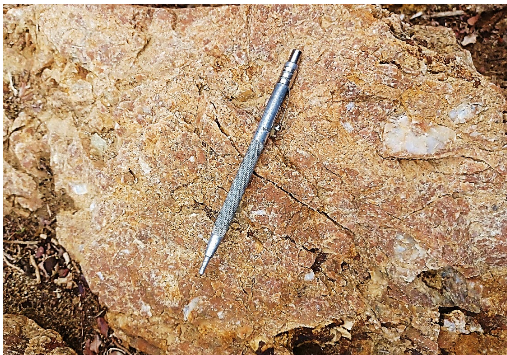
Figure 7: Silicified breccias identified at the T4 target area (refer ASX announcement 23 August 2022).
