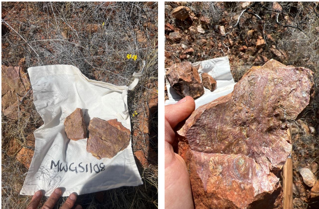
Figure 10: Massive monazite sample MWGS1108 (left) and MWGS0848 (right) which assayed 28.07% TREO with 4.63% Nd_2O_3 + Pr_6O_{11} and 23.81% TREO with 3.97% Nd_2O_3 + Pr_6O_{11} .
