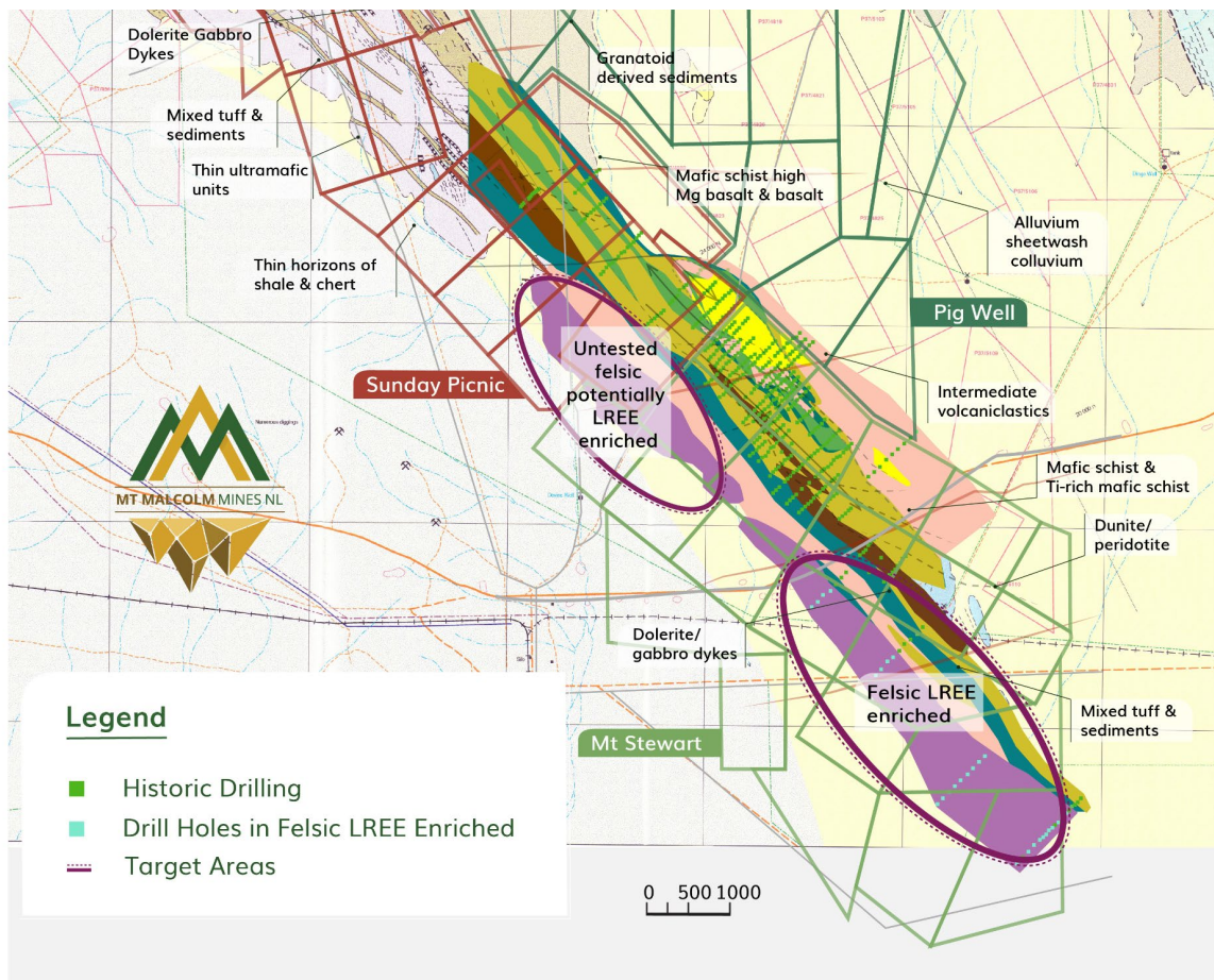
Fig: 15 Mt Stewart and Sunday-Picnic prospects with geology, historic drilling and REE target areas
