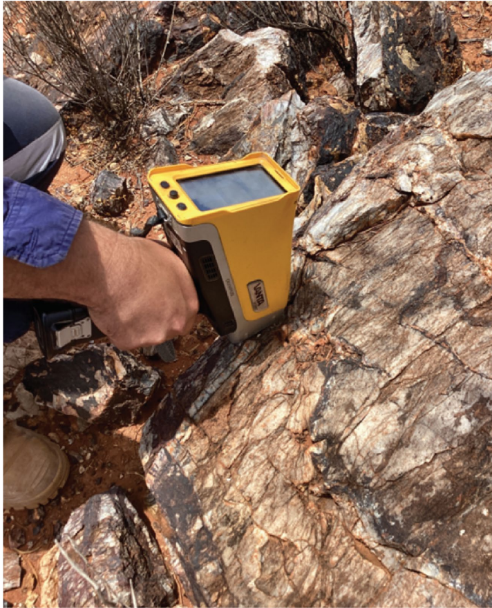
Fig 17: Chert horizon cut by felsic veins of magmatic affinity and the elevated pXRF gun results.
