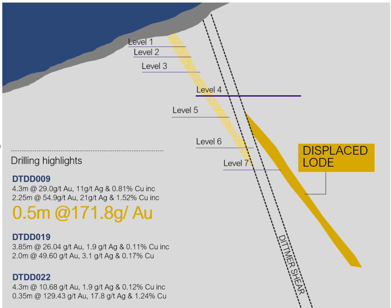
Figure 3. Drilling has confirmed that the main lode at the old Dittmer Mine has been displaced and continues less than 30m away from historic workings and existing underground access.
