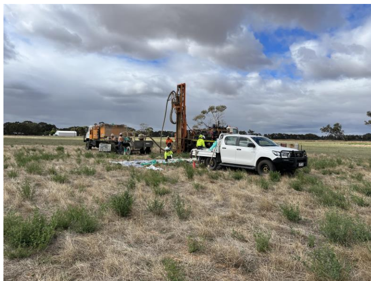
Figure 13 Aircore rig in the paddocks
