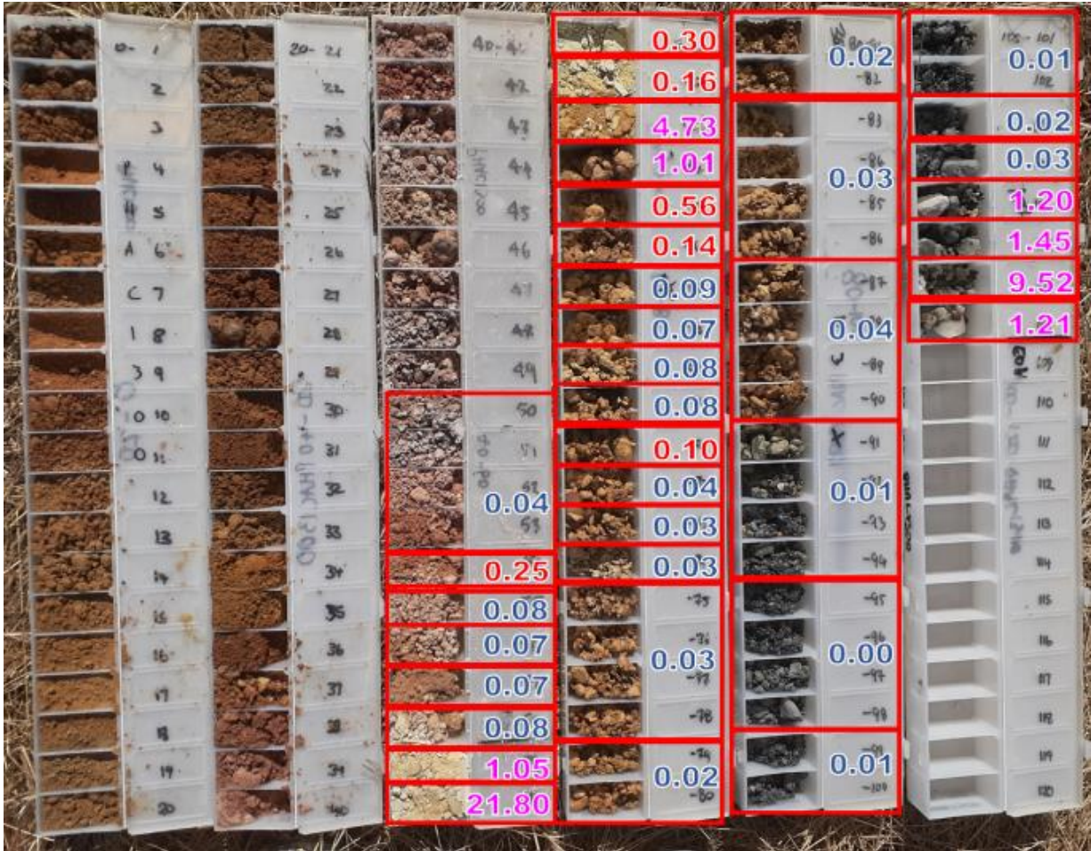
Figure 7 Chip tray photo of hole PHAC1300 showing the high-grade zones (g/t Au) in the saprolite, and in primary mineralisation at the base of the hole
