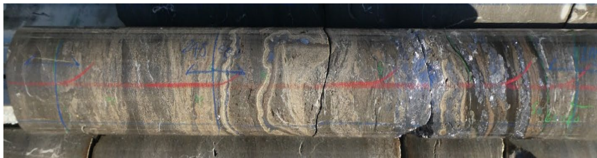
Figure 12: Close up photograph of drill core interval 245.3 m to 246.1 m showing colloform massive sulphides (low-iron sphalerite = cream coloured & galena = blue grey)
