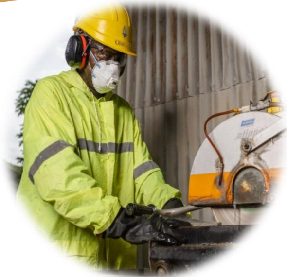
Staff Cutting Diamond Drill Core
