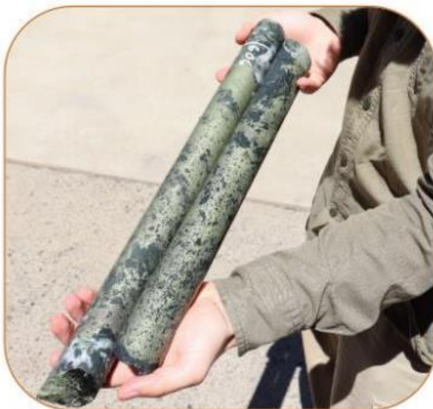
Figure 3: Semi massive chalcopyrite mineralisation in drill core from CANDD016C
