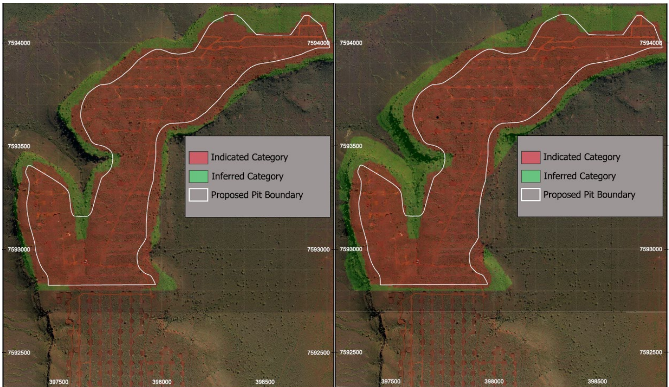
Figure 4. Plan view showing the classification of the mineralisation. Upper channel – left and lower channel – right (Indicated Resource – orange, Inferred Resource - green).
