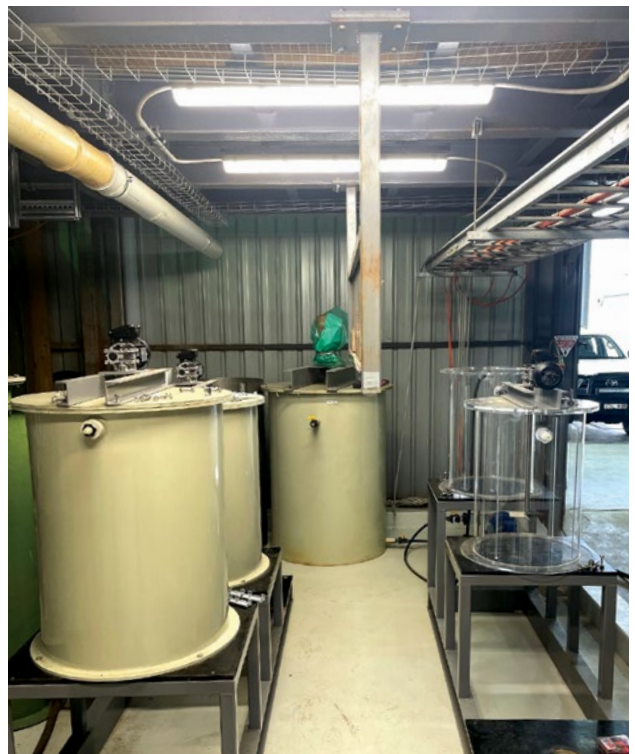
Figure 9 – Demonstration Plant. Left: Iron oxidation and precipitation circuit. Right: Installation of iron polishing and MHP precipitation circuits
