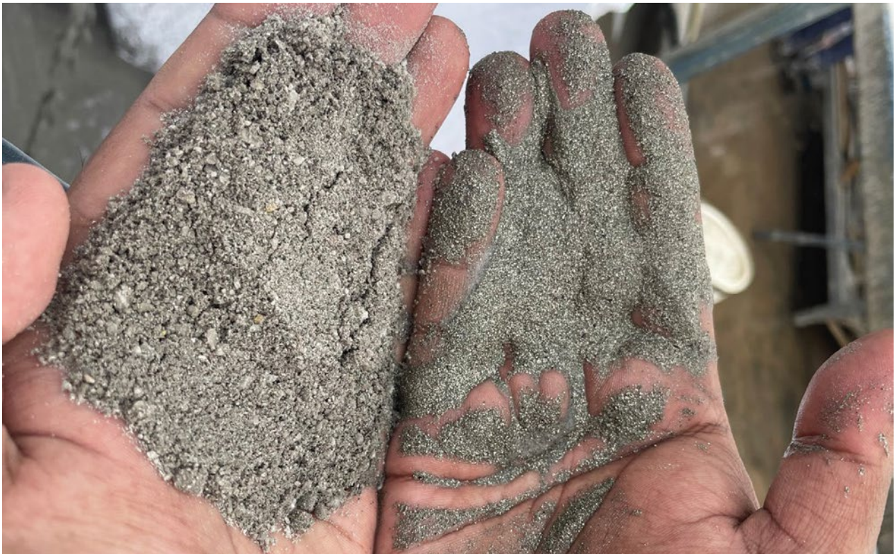
Figure 5 – Feed ore milled to <4 mm on left hand, and gravity concentrate on right hand
