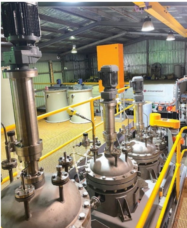
Figure 9 – Demonstration Plant. Left: Iron oxidation and precipitation circuit. Right: Installation of iron polishing and MHP precipitation circuits
