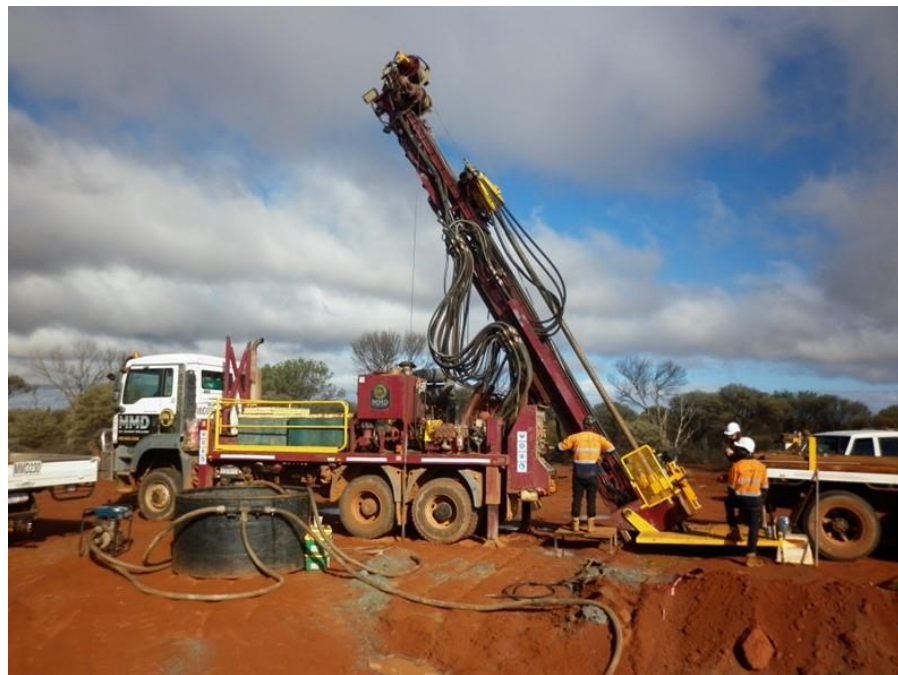
Figure 4 – Stage 10 diamond core rig drilling core tails
