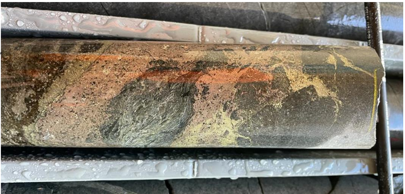
Figure 2: 22B2DD003 (26.8 -27.1 metre interval – NQ core 47.6mm diameter). 0.3m @ 4.14% Ni Eq Strongly mineralised dolerite with fine-grained pyrrhotite, chalcopyrite and coarse minerals of pentlandite. Mineralisation is semi-massive and interstitial. 1
