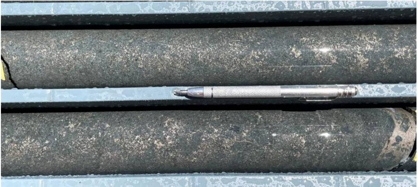
Figure 3: 22B2DD003 (40.2-42.0 metres – NQ core 47.6mm diameter) 1.8m @ 2.32% Ni Eq Strongly mineralised dolerite with disseminated angular blebs of fine-grained pyrrhotite and pentlandite with minor chalcopyrite. 1
