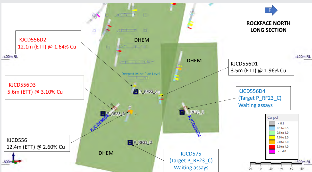
Figure 3: Longitudinal (plane-of-vein) projection of the lower part of Rockface North target between 750m and 950m depth showing the latest intersection in KJCD556D2 and KJCD556D3. An additional completed hole is awaiting assay (KJCD556D4). The target of the current hole (KJCD575) is shown. DHEM conductors are shown as green rectangles. Planned mine openings are also shown. All intersections are quoted as estimated true thickness (ETT).
