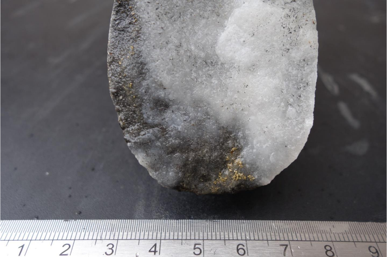
Figure 13: Visible gold is preserved as up to ~1cm sized aggregates made up of many less than 0.5mm grains within a ~1cm thick, translucent-white, drusy quartz veinlet at ~127.55m in UGA-52.
