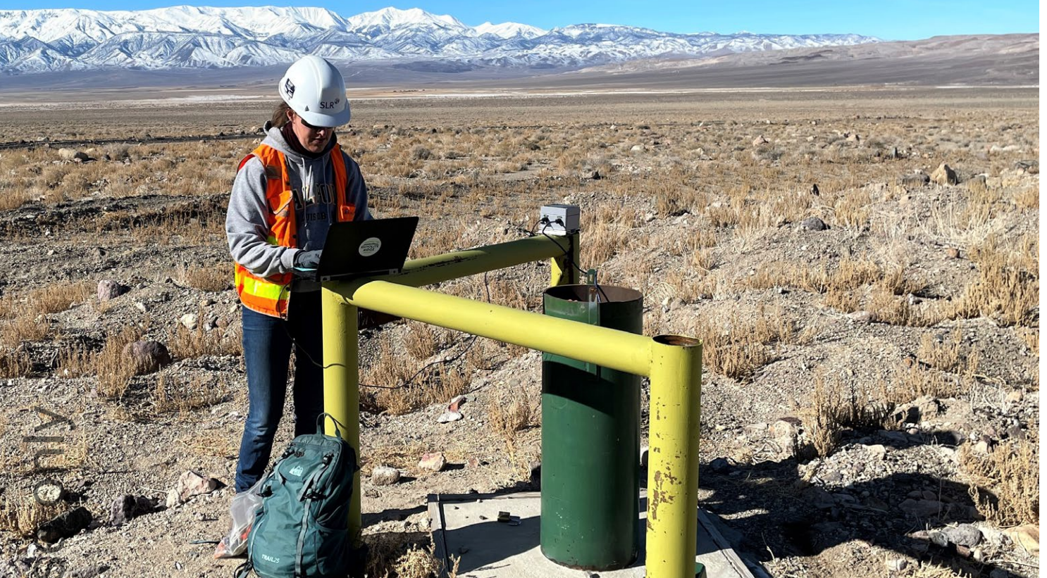
Preparation with Purpose: Collecting baseline groundwater data to set the stage for responsible mining.
