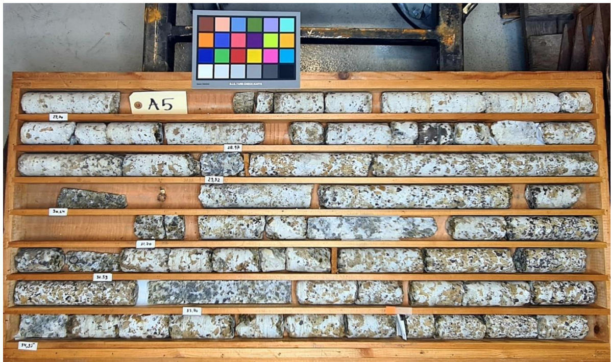
Figure 20: Diamond drill core from Hole A, upper zinc zone (approximately 26.8 to 35.2m down hole), showing siderite and sphalerite mineralisation in a quartz host with black marmatite, an iron-rich variety of sphalerite.
