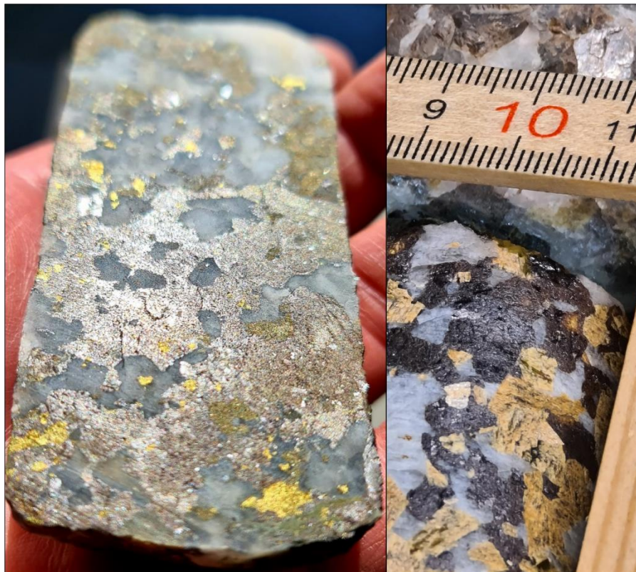
Figure 21: Left image: Half-core (width approximately 40mm) showing semi-massive marmatite (Mar), sphalerite (Sp) and chalcopyrite (Cpy) in a quartz (Qz) host. The piece of core shown is from the lower zinc-copper zone (86.2 to 89.9m), which has been visually estimated to consist of ~40% quartz (Qz) and ~60% sulphides with the sulphides comprising ~40% sphalerite, ~5% marmatite and ~5-10% chalcopyrite. The balance (~5-10%) is comprised of sulphide minerals that are too small to positively identify. Right image: Drill core showing semi-massive, coarse-grained siderite (Sid) and marmatite (Mar) in a quartz (Qz) host. The piece of core shown is from the upper zinc zone (27.15m to 39.85m), which has been visually estimated to consist of ~50% quartz, ~40% siderite and ~2 to 10% sulphides with the sulphides almost exclusively comprising of marmatite.
