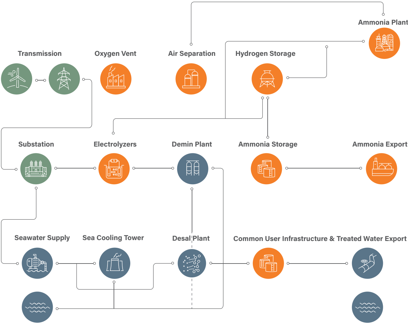
Upstream power and Cape Hardy green hydrogen precinct anhydrous ammonia block flow schematic (source AMP Energy).
