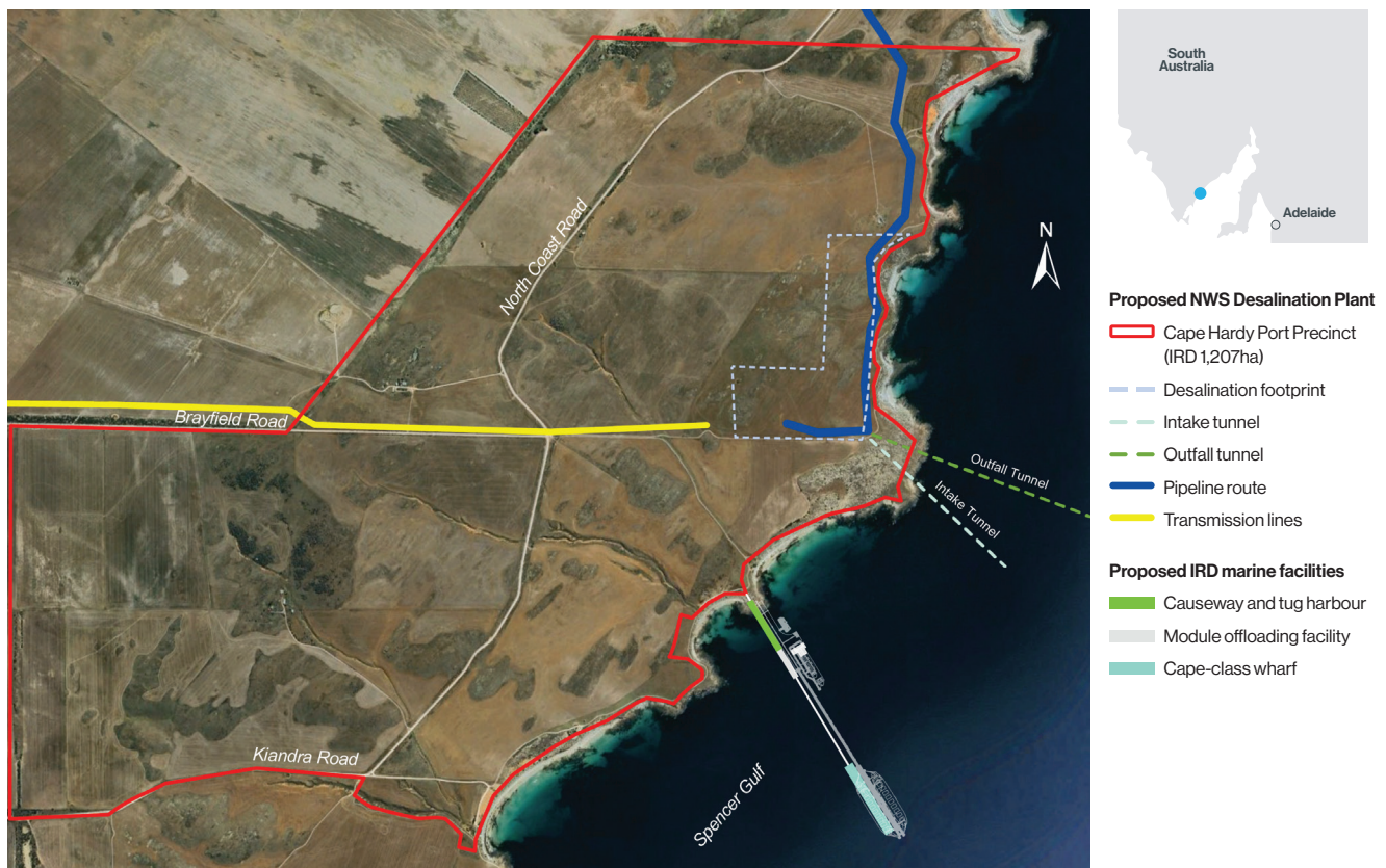
Iron Road and Northern Water Supply (NWS) Cape Hardy Spatial Reference – Preliminary site plan for proposed desalination plant
