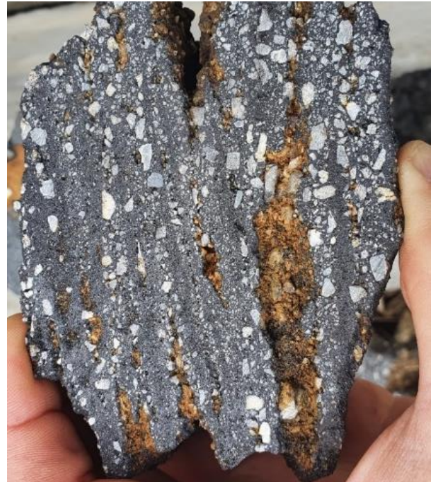
Figure 4 | Surface sample of cobalt enriched, manganese replacement rock returning 1.19% cobalt, 0.24% nickel and 13.4% manganese.
