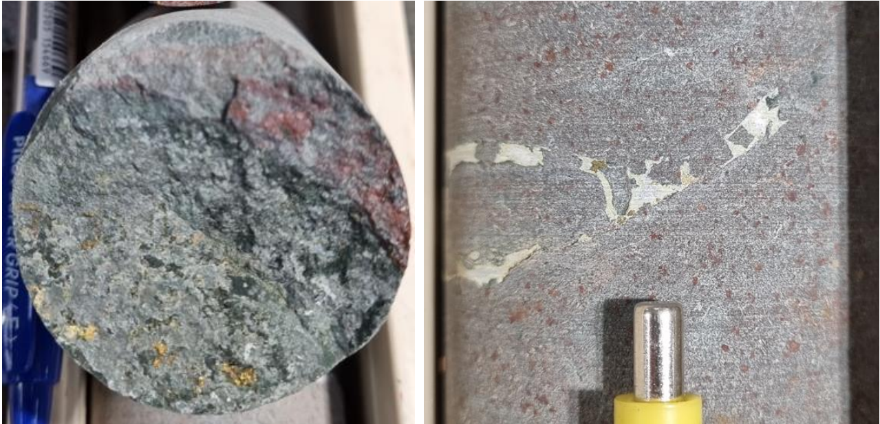
Figure 10 – Left –Chalcopyrite on fracture surface. Right – Tarnished chalcopyrite in carbonate filled fracture. Core from Sample ID 610027
