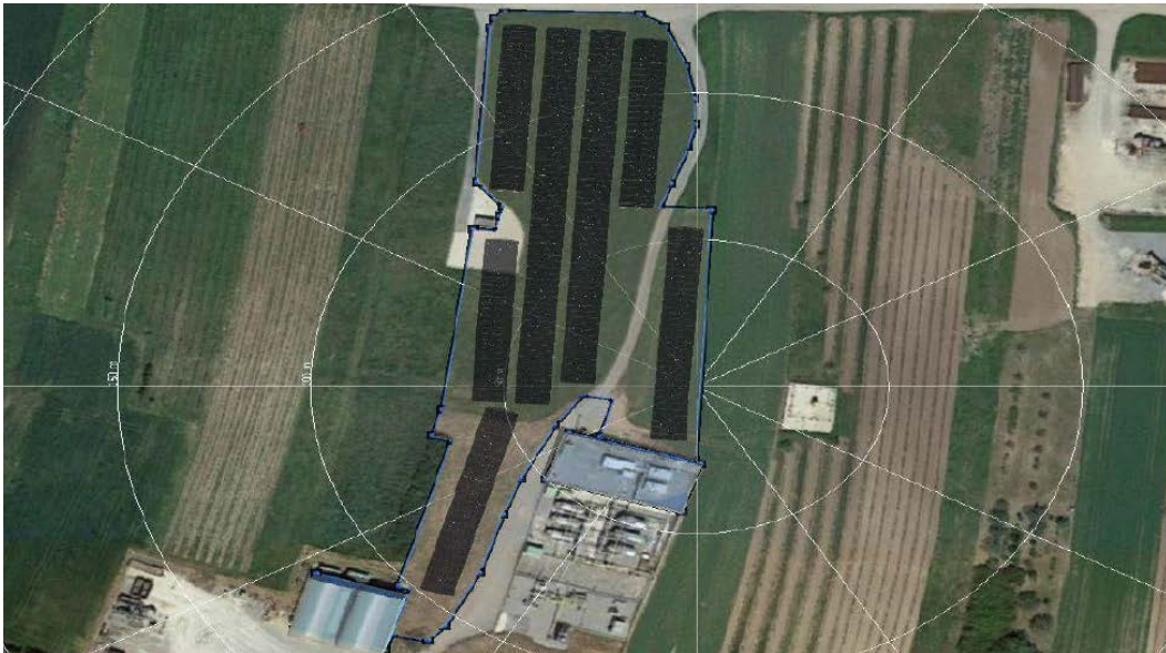
Figure 7: Potential layout of the PV panels at the Gaiselberg site (approx. 1 MWp)
