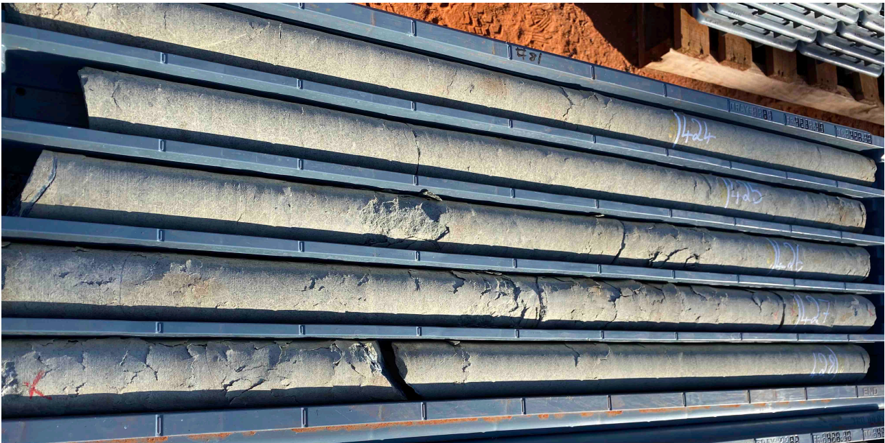
Figure 1B: Mulga Tank Hole MTD020 Tray 81 423m to 428m 7 August 2022 Uncut core beginning to show spalling within 3 weeks of being drilled
