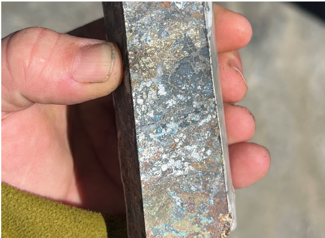
Figure 4: 2022-KNG-013B returned 0.24m @ 130g/t Au, 732g/t Ag and 28 % Pb, 0.40 % Zn from 21.0m. Mineralisation characterised by a massive sulphide vein with galena, pyrite and sphalerite.
