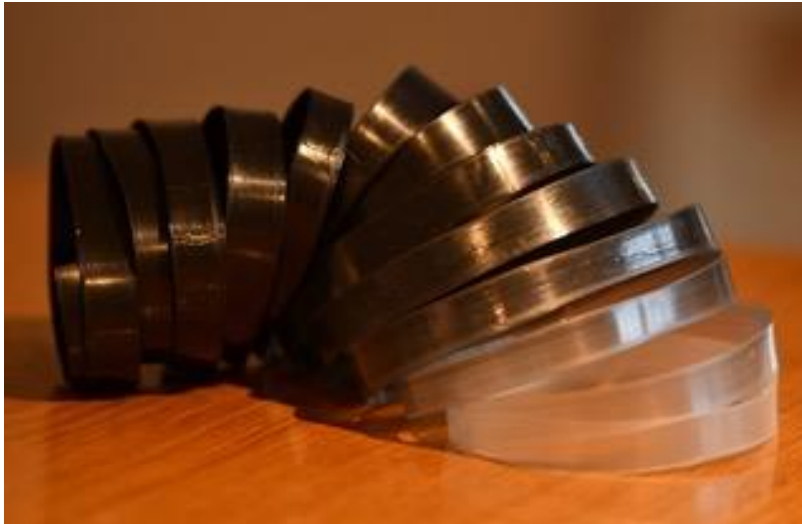
Polymer tape with progressively higher percentages of CNT added
