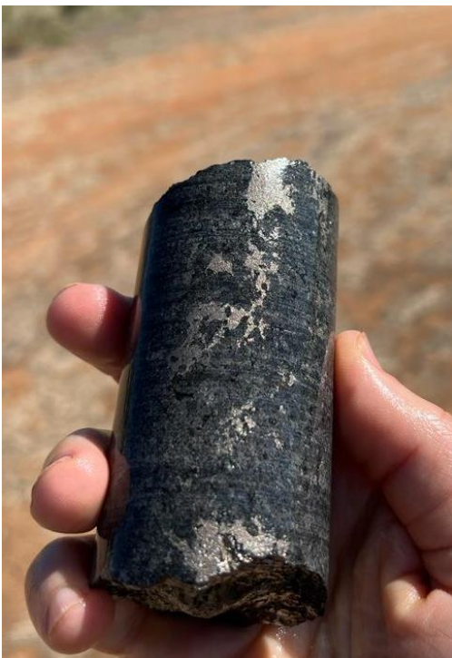
Figure 1. Nickel-Copper sulphides in Diamond drilling from the first hole at Bow River Project at 368m depth.
