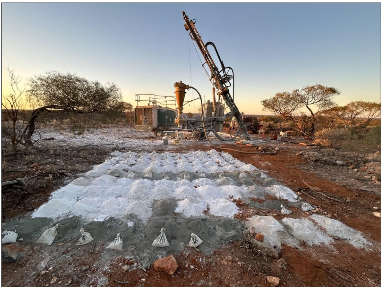
Figure 4: RC drilling at Mt Edon (hole MD23- 07) indicate thick zones (white samples), view to west
