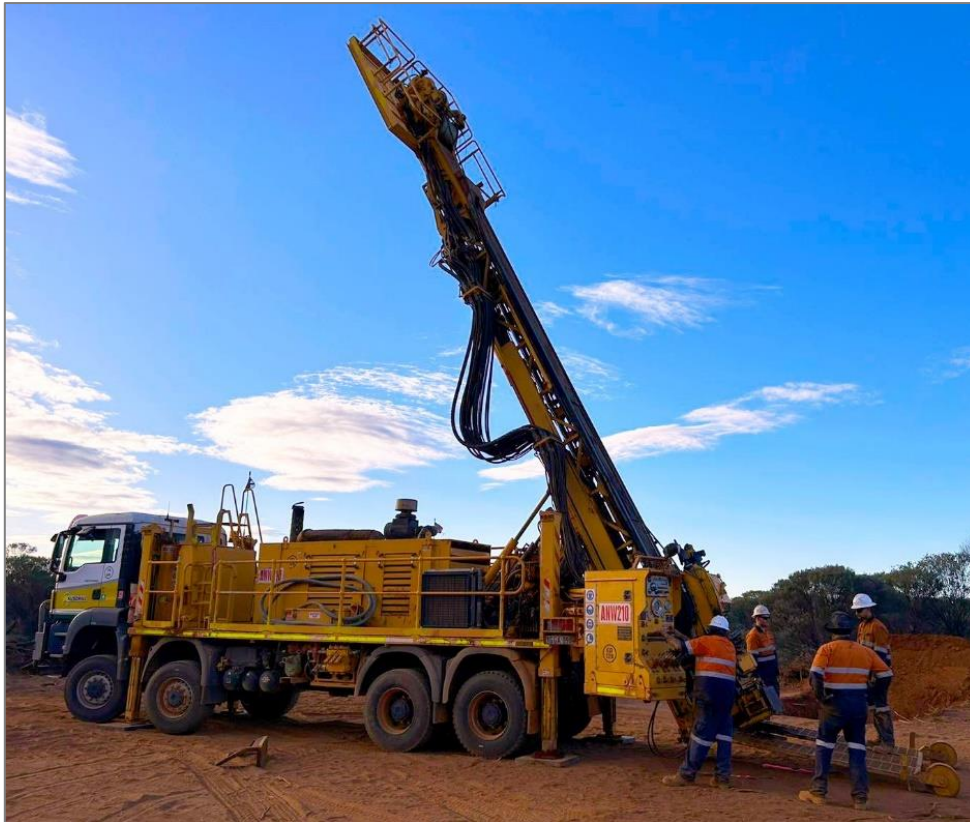
Figure 2: Diamond drilling at Revere Gold Project
