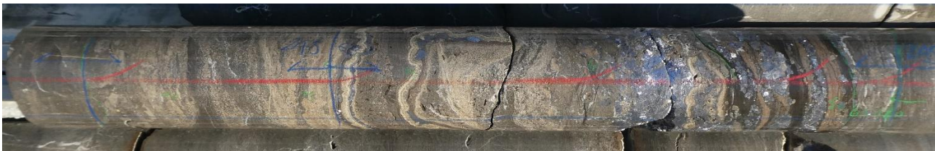
Figure 6 Close up photograph of drill core interval 245.3m to 246.1m showing colloform massive sulphides (low-iron sphalerite = cream coloured & galena = blue grey)
