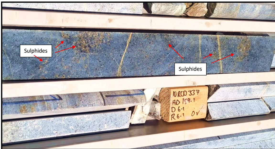
Figure 11 — Diamond drill core from metallurgical hole NRCD337 at 158m down hole showing bands of disseminated sulphides. Typical disseminated sulphide abundance over one metre mineralised intervals is 5% or less. Field of view is approximately 40cm across. Sulphide interval shown is within the 34-metre significant interval.
