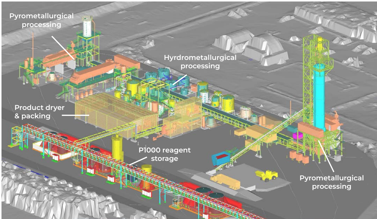
Figure 10: Proposed Mid-Stream Demonstration Plant schematic
