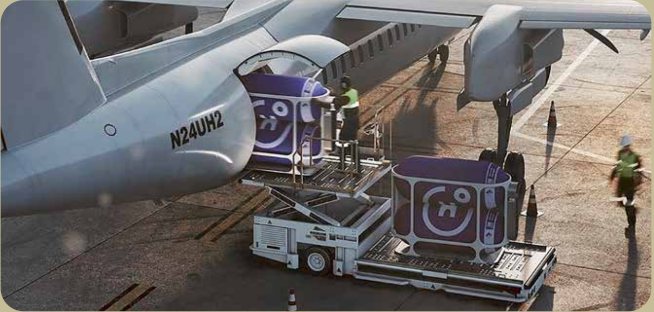
Converted aircraft being refuelled with hydrogen storage capsules. Image courtesy of Universal Hydrogen (2022).
