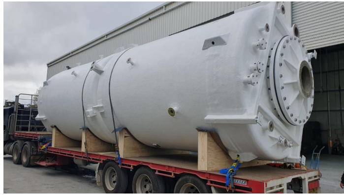
Figure 1 Equipment for vanadium electrolyte production – L-R bag unit and electrolyte tank
