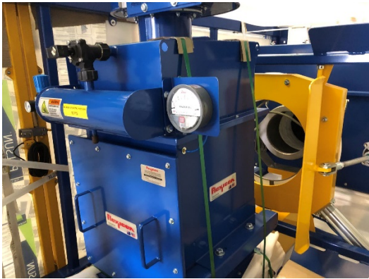
Figure 1 Equipment for vanadium electrolyte production – L-R bag unit and electrolyte tank
