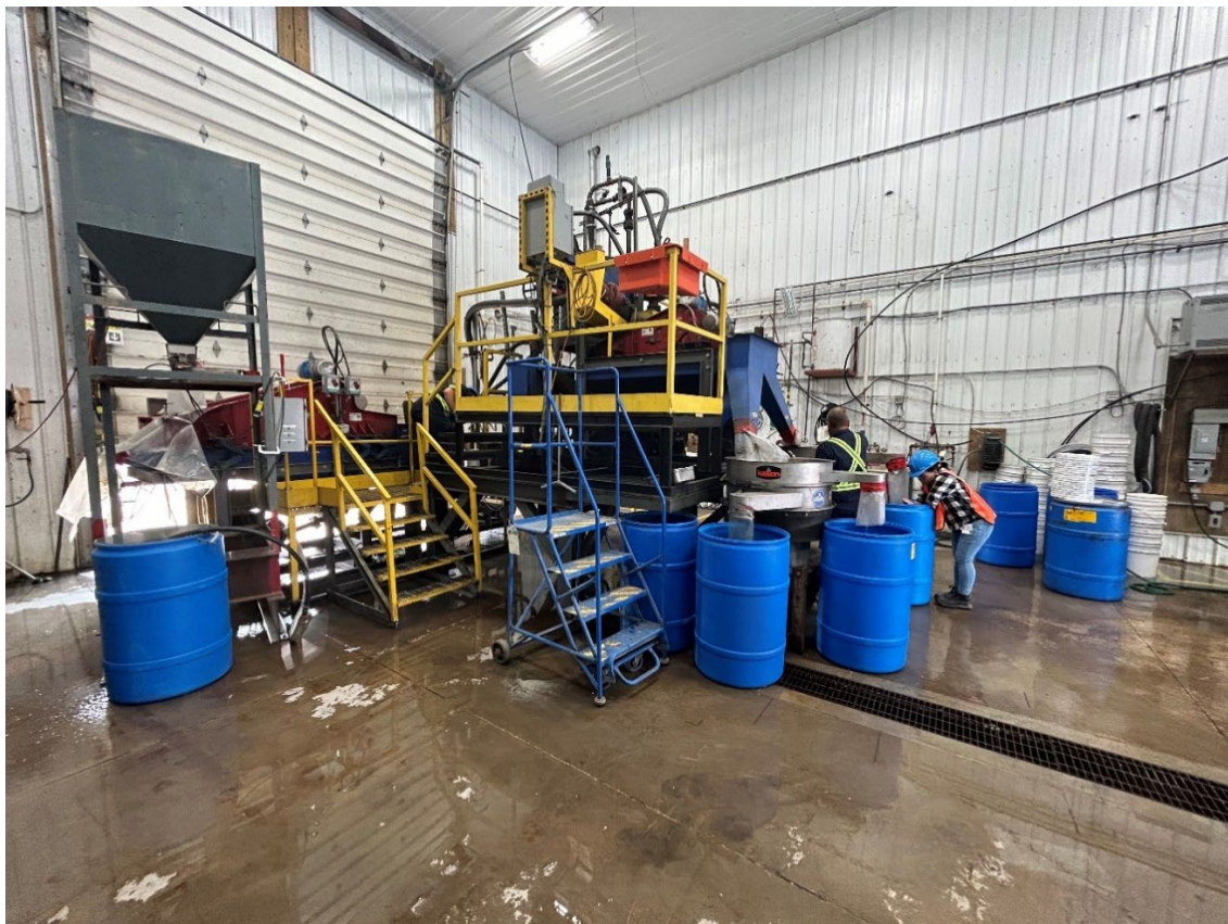
Figure 2. Dense Media Separation (DMS) Pilot Plant located at SGS' Lakefield, used for the Colina DMS testwork.
