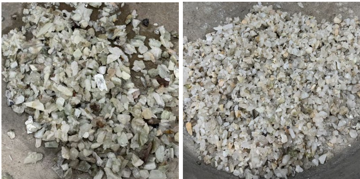
Figure 1. Colina composite 1 indicating 6.3mm (+1mm) sink (left) and float (right) results produced from DMS test work on the Colina ore samples.
