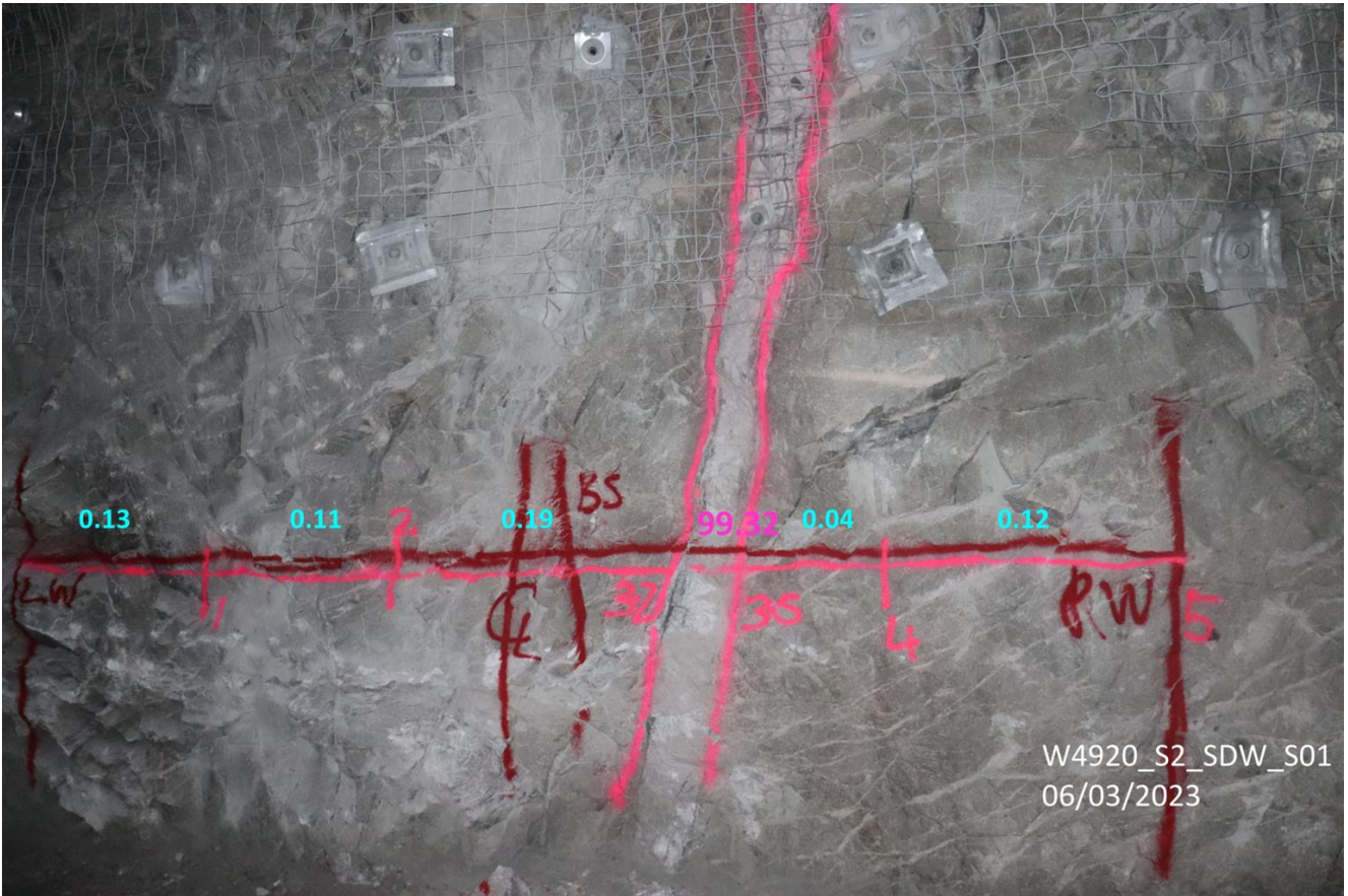
Figure 10. Development along the W4920m south following high-grade tension veins, face grade 10.47g/t and the high-grade vein was 99.3/t.
