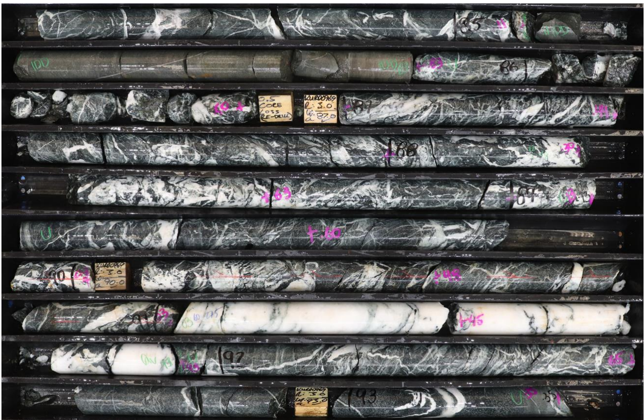
Figure 7. Core photographs of KHRD0969 showing intense mineralisation within the ultramafic footwall.
