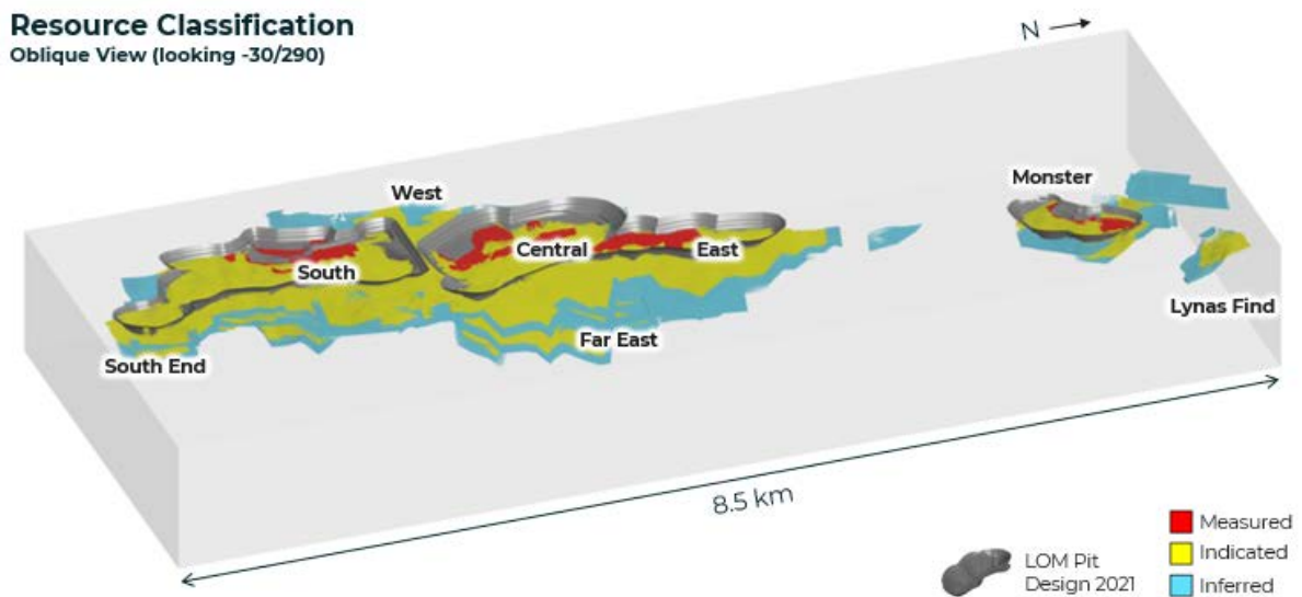
Figure 4 – Oblique View (looking -30/290) showing mineralised domains (pegmatites) and 2021 LOM pit designs
