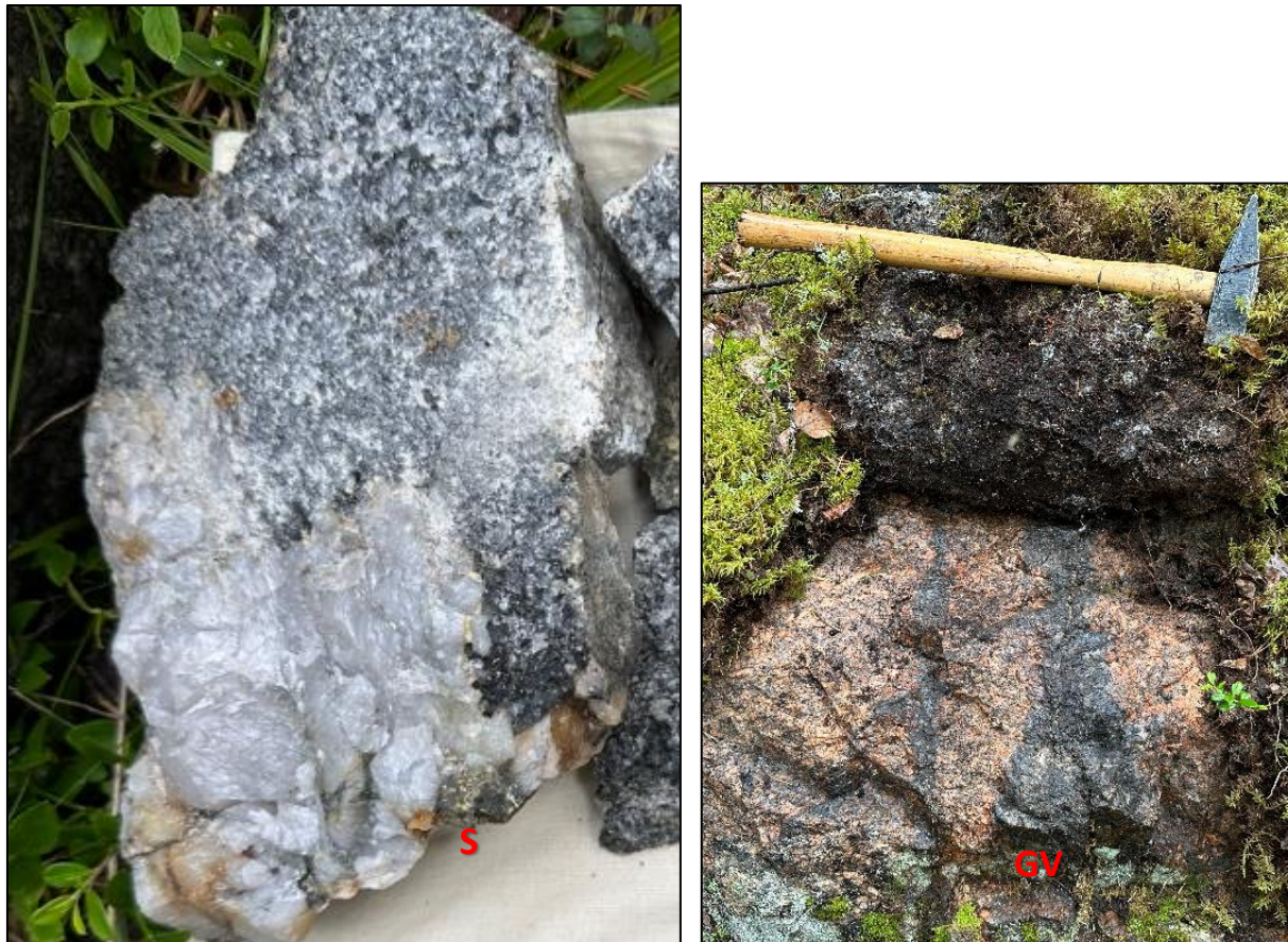
Figure 4: (Left) Photograph of altered possible granite greisen dominated by quartz, topaz and dark mica with minor chalcopyrite-pyrite-sphalerite sulphides (S) in quartz veins (Sample KUSGS38), and right coarse red K feldspar-albite-hematite rapakivi granite host and sheeted greisen veins (GV) with fluorite up to 20cm. (Sample KUSGS42). Clear evidence of fluorite is highlighted in Figure 5.
