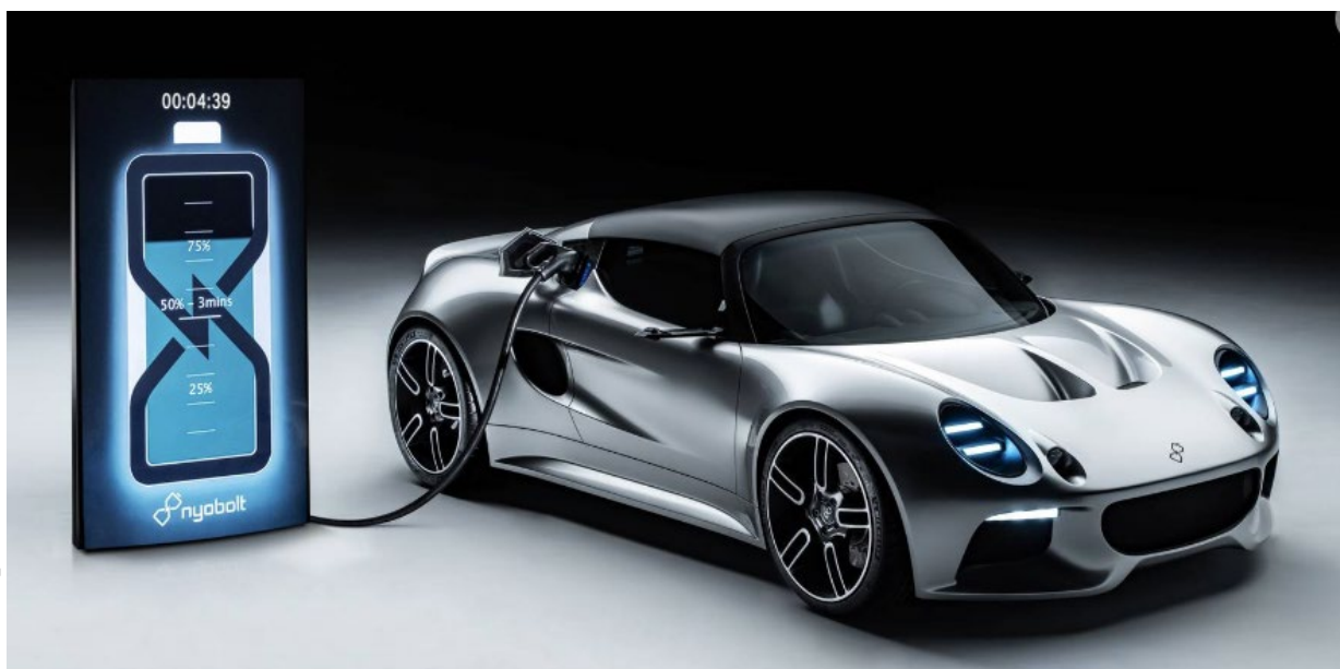
Figure 4. The 35kWh battery pack gives the Elise-based Nybolt a range of up to 250km on one charge
