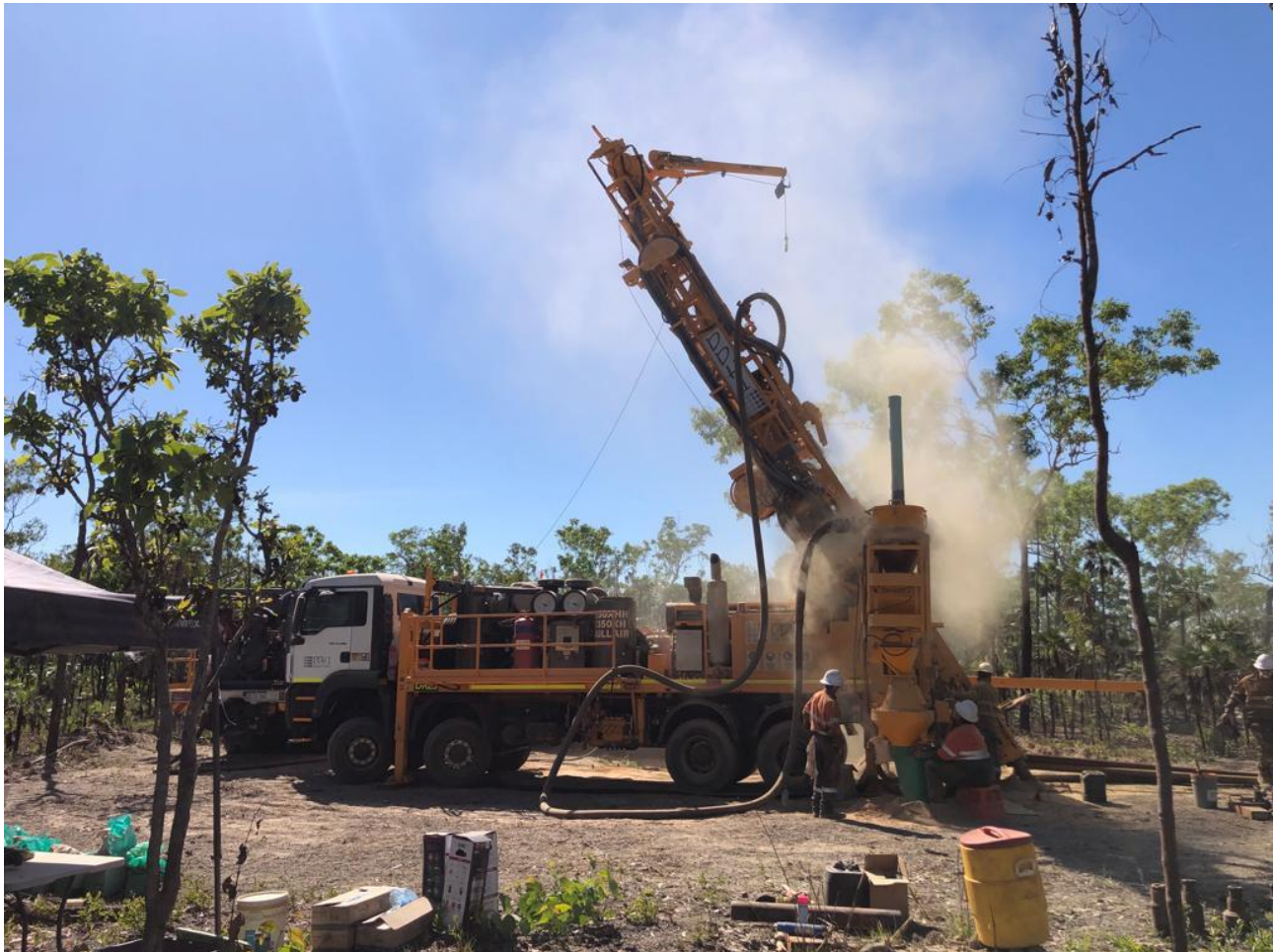
Figure 1: Dual RC/DD rig in operation at Perseverance Prospect, Kings Landing Area
