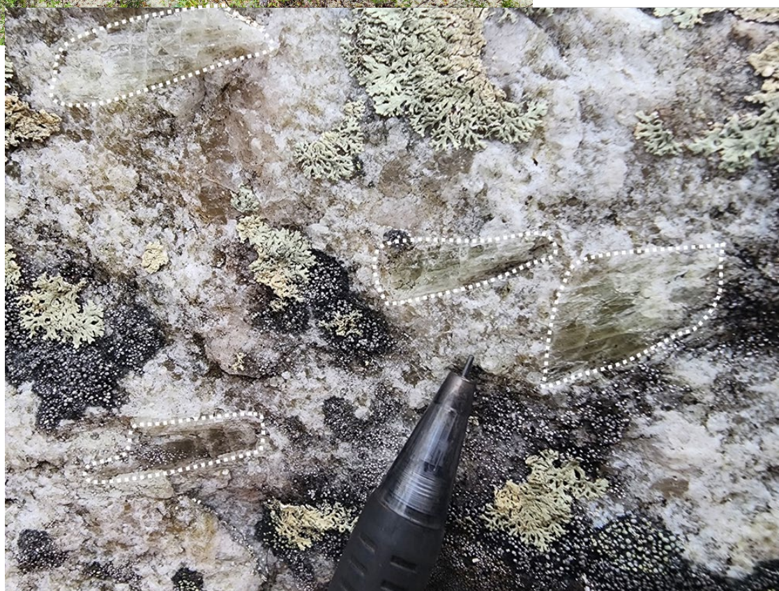
Figure 2: Cygnus Business Development Manager and Geologist, Gareth Reynolds, inspecting a large spodumene-bearing pegmatite boulder. Close up of spodumene mineralisation (spodumene crystals circled in white). Sample ID 155790004* (refer CY5's ASX Announcement dated 12 July 2023).
