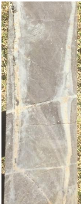
Figure 4 Core from Hole TOR001C showing lithium rich metasediments at 7.8m depth.. Grade 0.35% Li2O based on the assays received.
