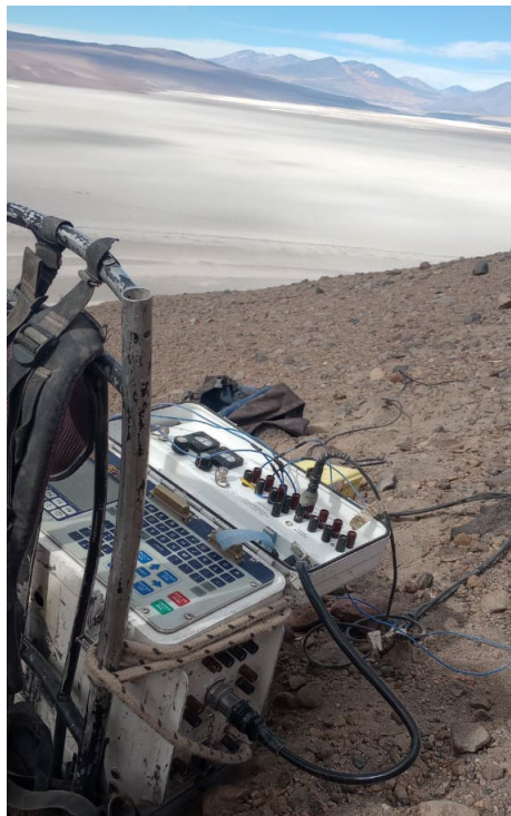
Figure 1 – Quantec CSAMT equipment on site at the Rio Grande Sur Lithium Project
