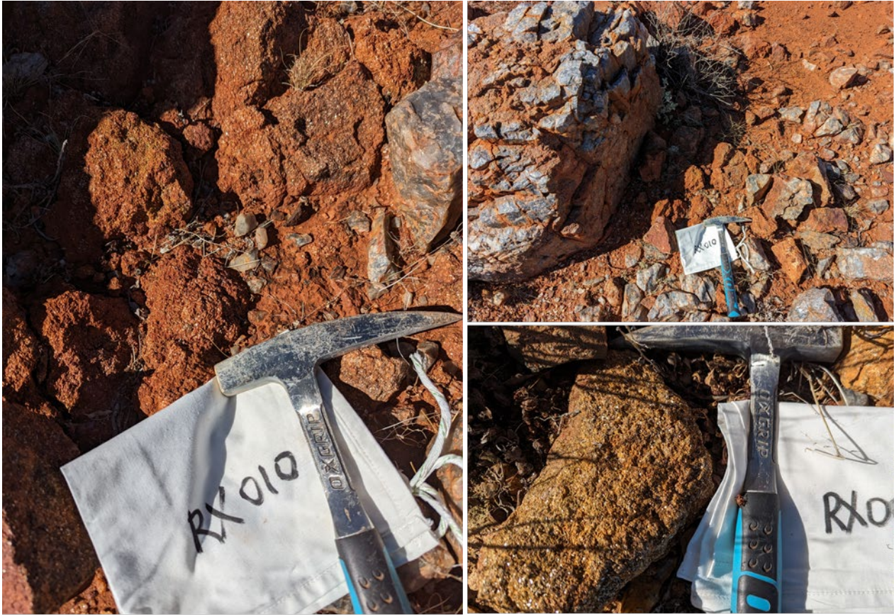
Figure 3: Photographs of mica dominant greisen rock samples taken from over the Loader Prospect.
