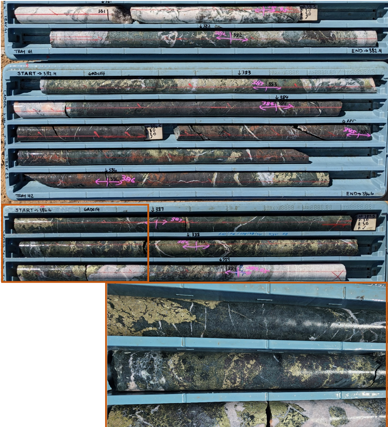
Figure 4: Zone of visible high-grade sulphide mineralisation intersected at target depth, correlating with significant downhole intercept of 7.05m @ 2.23% Cu from 382.00m (inset view on right).
