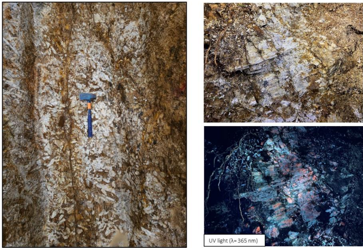
Figure 4: UV fluorescence spodumene crystals within the Trench 2 pegmatite – spodumene minerals are white to cream coloured minerals within the host pegmatite unit.
