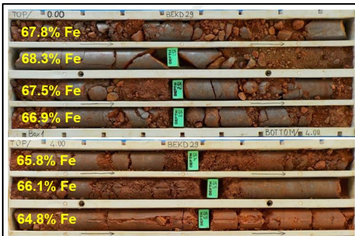
Photo 6.2: High-Grade Iron Mineralisation BEKD029
