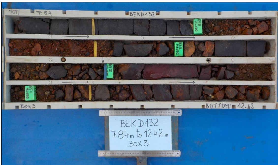
Figure 7.8: Photograph of Wet Half Core From BEKD132 After Being Sampled.
