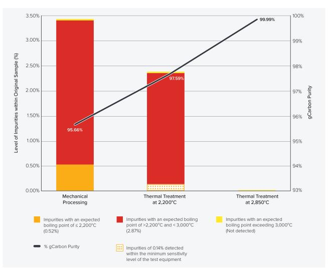
The final phase of the thermal treatment was conducted at a temperature of 2,850°C under substantially similar conditions to that of the first phase program. The result of the thermal treatment of Uley flake at this temperature achieved a near imperfect IER and a purity of Uley flake of more than 99.99%. The chart above graphically illustrates the results of the first and second phases of the thermal treatment testwork program.
