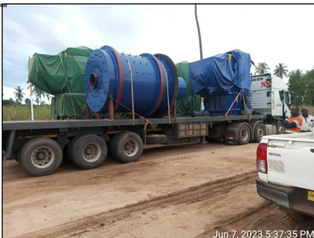
Figure 2: Drum Scrubber and attritioning mills on site (left) and two sections of the rotary drier in temporary laydown near the mounting plinths (right).
