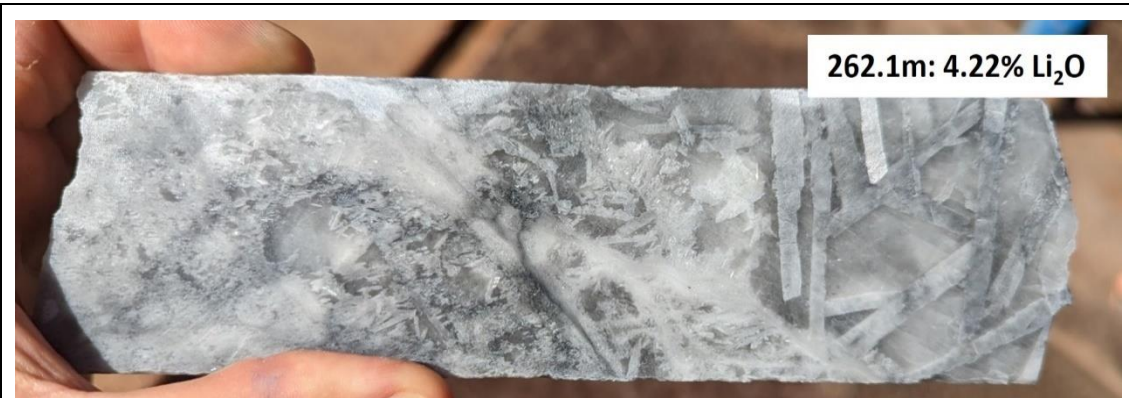
Image 1: Abundant coarse-bladed spodumene (elongate white-light grey crystals) hosted in grey quartz in hole ANDD0208 with downhole depths and lithium grades
