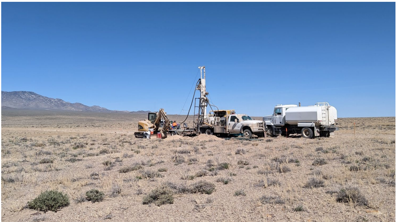
Figure 3. Photograph of air core drill rig set up over drill hole PL04.
