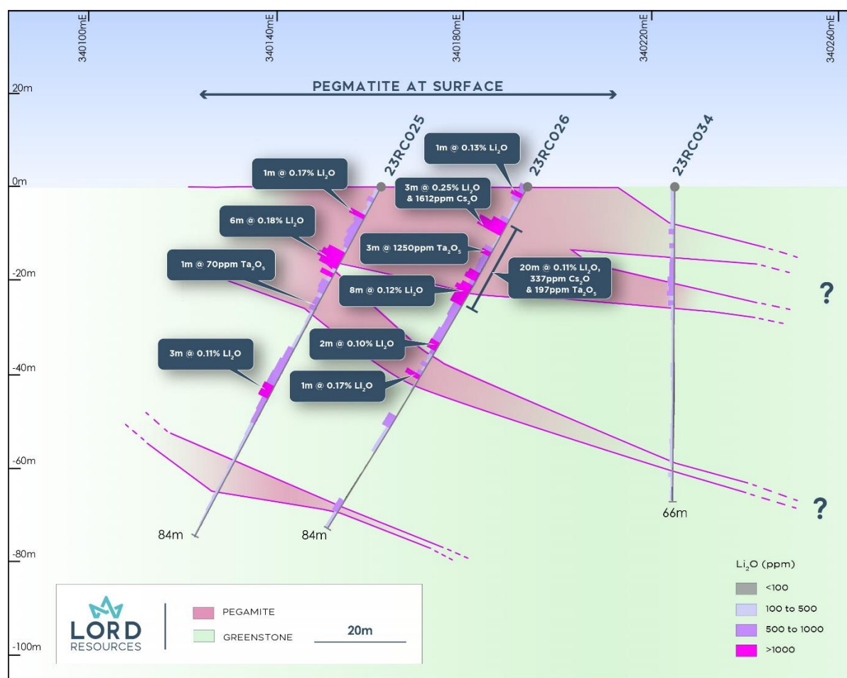
Figure 4 - Cross section from 6558750mN, showing zoned pegmatite in 23RC026.
