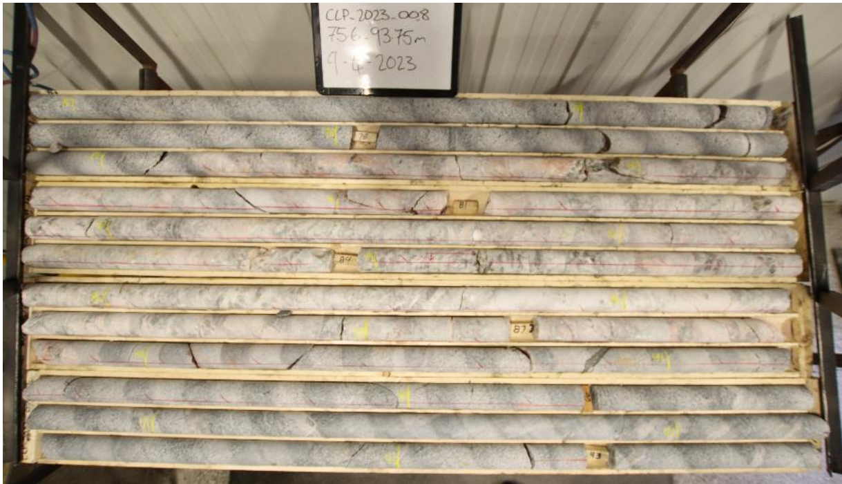
Photos 3. Chubb diamond drill hole CLP008 which intercepted 8.74 m of large crystal structure of the spodumene-bearing pegmatites from 79.14m depth with an estimated 10 to 30% spodumene content 9 .
