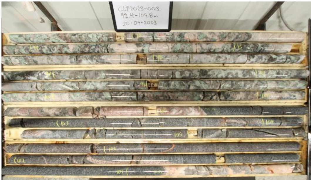
Photo 5: Chubb diamond drill hole CLP003 which intercepted 12.22 m of large crystal structure of the spodumene-bearing pegmatites from 90.00m depth with an estimated 10 to 30% spodumene content.
