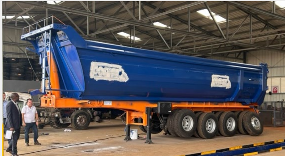
4-axle, 50 t payload trailers being assessed
